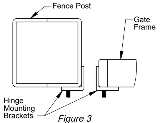
③ Install self-closing hinge assembly to mounting flanges installed in Step 2, and secure with washers and acorn nuts (USING HAND TOOLS ONLY). Hinge should be positioned as shown so that the locking grooves on the mounting flanges will align with grooves on the back side of the hinge assembly (Figure 5).
